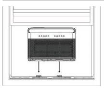
A. Set the air conditioner on top of the support bracket. Ensure the grooves on the bottom of the air conditioner align with the Main Supports. Using a level, check for proper tilt towards the outside.
