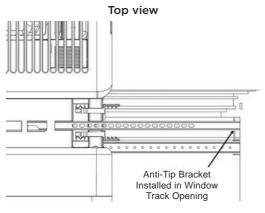
The images to the left show what a properly installed Anti-Tip Bracket into the window track should look like.
