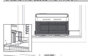
D. Measure the distance between the Side Arm Hinge and the closest part of the window frame in line with the Side Arm. Add 1/4" to this distance and cut the Side Arm Foam to length.
