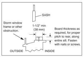
Add wood as shown, or remove storm window before air conditioner is installed.
