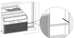
The images to the left show what a properly installed Anti-Tip Bracket into the window track should look like.
