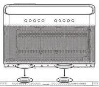
Pull the window down into the slot to help align the unit in the correct location. Keep the window partially inserted into the window slot to help support the air conditioner during installation.
