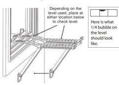
B. Move the Angled Support Arms toward the exterior wall until the Angled Support Feet touch the wall. Place a level on a flat area of the bracket and adjust the Angled Support Arms so the bracket is tilted downwards toward the outdoors to allow condensate to drain out. The proper angle is when the level reads 1/4 bubble (reference image for 1/4 bubble).
