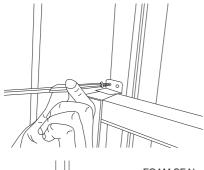
To secure lower sash in place, attach right angle sash lock with 1/2" Type A Screws as shown.
