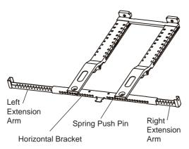
On a flat surface such as a table press the spring push pin and adjust the Left Extension Arm to the Left side of the Horizontal Bracket
