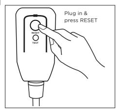
The power supply cord contains a current device that senses damage to the power cord. Test your power supply cord as follows:
