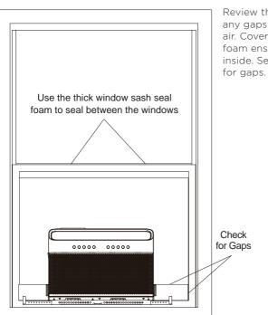
Review the installation and check for any gaps or openings to the outdoor air. Cover these gaps with the provided foam ensuring no outdoor air leaks inside. See image for areas to check
