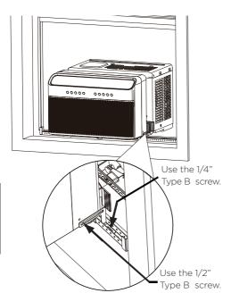
C. You must install the Open Window Brackets using the provided screws shown here.
