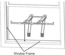
A. Before placing the bracket in the window, allow the Angled Support Arms to rotate down and make sure they don't fall out of the Main support arms. Place the support bracket assembly in your window opening on the bottom windowsill. The Horizontal Bracket and Extension Arms must be located on the indoor side of vour window frame.
