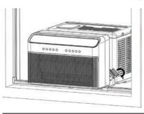
B. Fold both Side Arm Hinges down and measure the distance between the Side Arm Hinge and the Window Frame.
