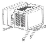
F. Close the window and extend both window locks located in the window slot to prevent the window from opening. Be sure to fully extend the locks so that they come in direct contact with the window.
